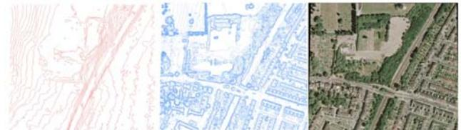
The data has been provided by InfoTerra and BlueSky, revealing their capability to build complex terrain and contour maps using LiDAR imagery plotting both the underlying ground contour (with buildings and vegetation removed) and a more complex image showing the contours with them in place (blue outlines).
